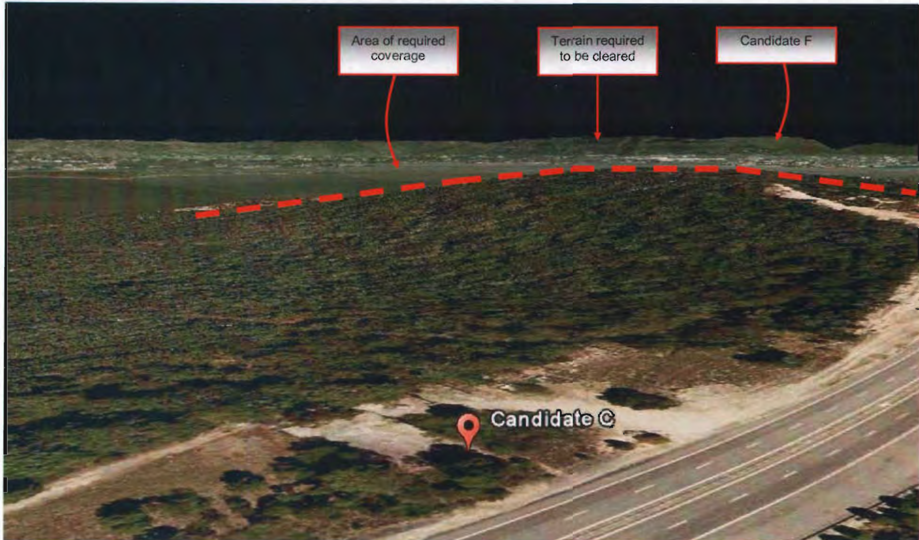
Figure 4- Google Earth image showing the terrain constraints blocking the target coverage from candidate C
